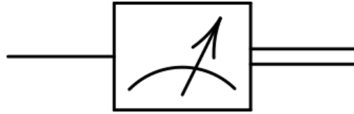
Figure 1.8: Circuit diagram of measurement. The two lines on the right hand side represent a classical bit.
