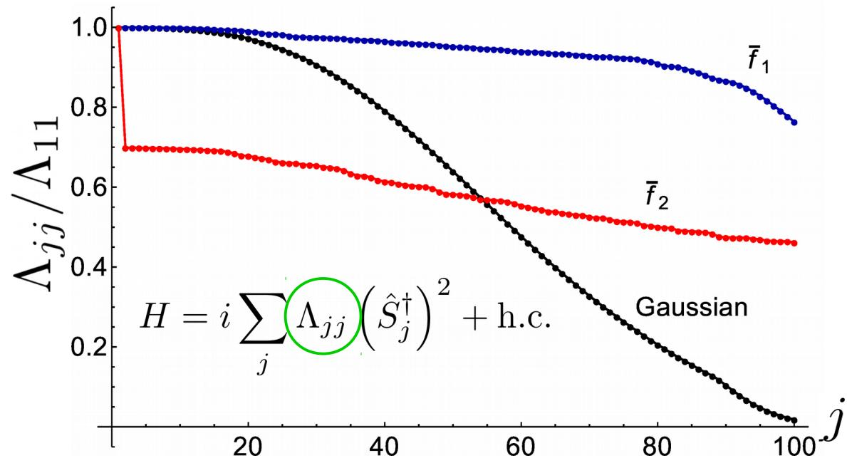
Adjust the squeezing spectrum :
